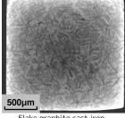
Flake graphite cast iron (No line hardening treatment)
