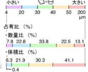
Color-coded by the effective diameter: Classified as the converted diameter of the sphere that each particle extracted from spherical cast iron
