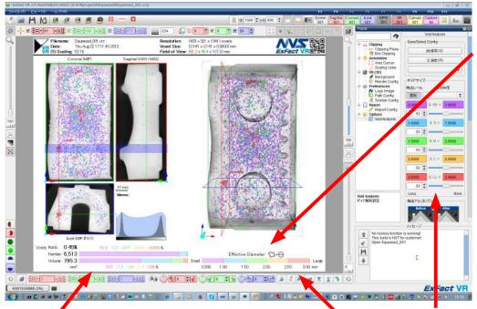
All voids have irregular shape convert as sphere then classify diameter of the sphere into 5 phases and display in different colors.
