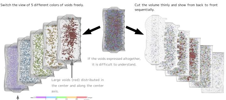
Large voids (red) distributed in the center and along the center axis.
