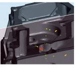
Automatically extract defects and particles existing inside the 3D images of casts and resin products. The extracted defects are presented in different colors.
