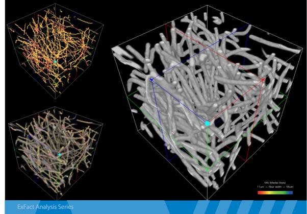
Imaging technologies such as X-ray CT, CLSM and TEM tomography provide a series of tomographic image of industrial products and materials for the construction of their 3D images ExEact® Analysis a software based on the novel concept of "Medial Axis" to capture the complex structure of various objects, offers a tool to conduct statistical evaluation/analysis on the properties of those 3D images, including shapes/distributions of grains/voids, as well as orientations of fibers.
