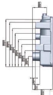
CAD-like 3D measurement based on 3D measurement data.
