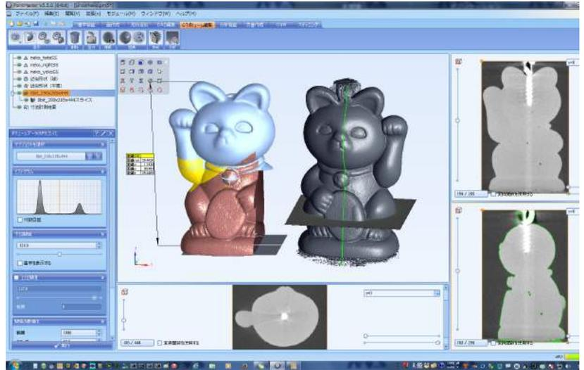
The CAD Link function offers an easy way to use 3D measurements data in various other fields including CAD, CAM and CAE. It allows users to construct surfaces on a polygon data or approximate it to a combination of shapes such as a plate or cylinder, with the resultant data provided as IGES or STEP files to be used in 3D CAD software.
