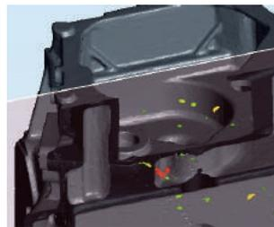
Automatically extract defects and particles existing inside the 3D images of casts and resin products. The extracted defects are presented in different colors.
