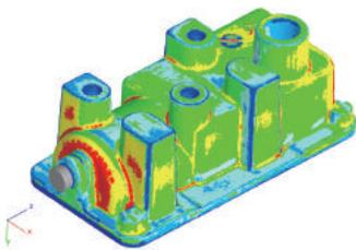
Position and align two different data sets for comparison, for example, between CAD data and measured data, or between two measured data sets.
