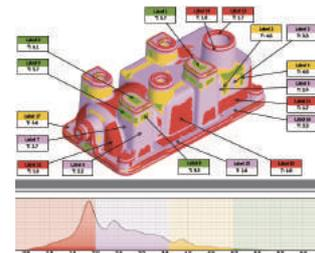
Detect the areas of a specified thickness and display them in different colors. Useful in evaluating the shape based on thickness.
