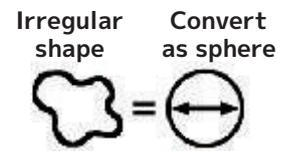
Called Effective Diameter is a concept commonly used in the industry of material science. The reason why not classified and displayed as volume, it is difficult to understand because the volume is a cubed numerical value and also tend to be biased towards to one side.
