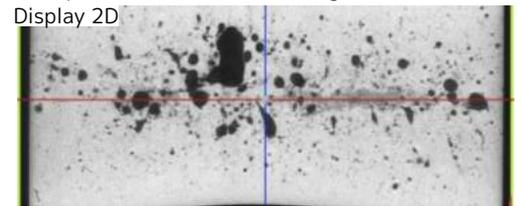
The image is constructed for understanding distribution of void's shape and features. It is a characteristic of ExFact VR that **express sharp rendering of contour** even on semitransparent display. By high level of interpolation processing, it express smooth even less than one pixel (sub pixel).
